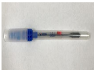
1. ATP Water Test Swab equilibrium
