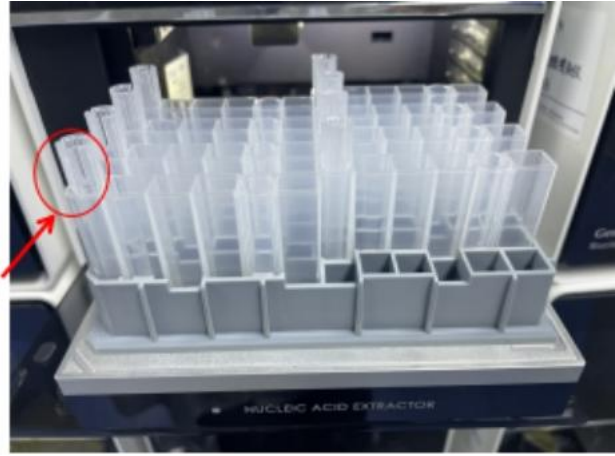
Figure 4. Put the single kit docking into the instrument
