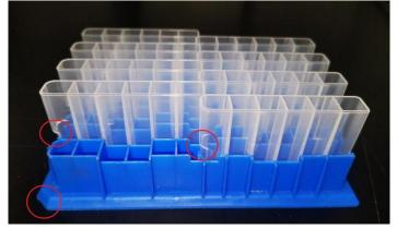
Figure 2. Put the 6 strip tube on the singe kit docking
