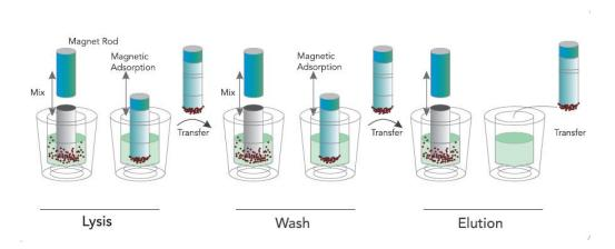
Figure 1. Schematic Diagram of Automatic Nucleic Acid Extractor
