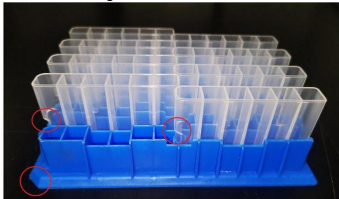
Figure 2. Put the 6 strip tube on the single kit docking
