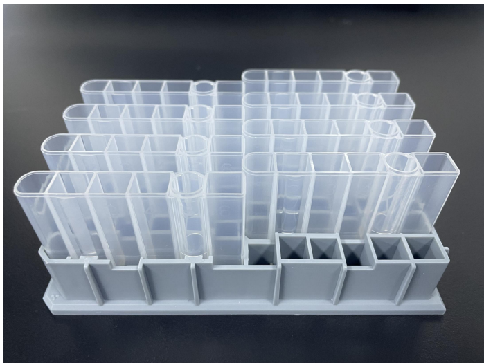
Figure 2. Put the 6 strip tube on the single kit docking
