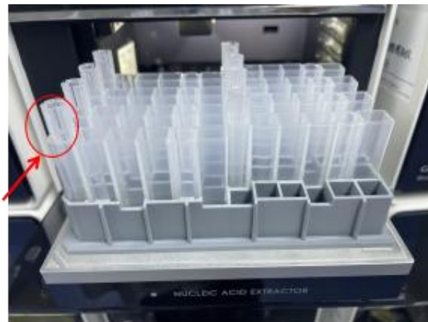
Figure 5. Put the single kit docking into the instrument
