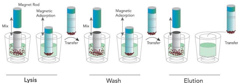
Figure 1. Schematic Diagram of Automatic Nucleic Acid Extractor
