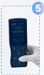
Press "OK" to start measurement
