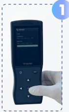
Select in turn "Setting"- "Help"- "Calibration"
