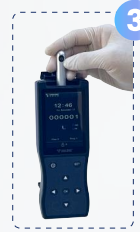
Insert EternalLight-H into Biolum
