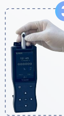
Insert EternalLight-H into Biolum
