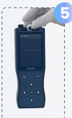
Insert EternalLight-H for calibration
