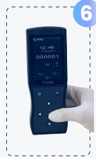
Press "OK" to start measurement
